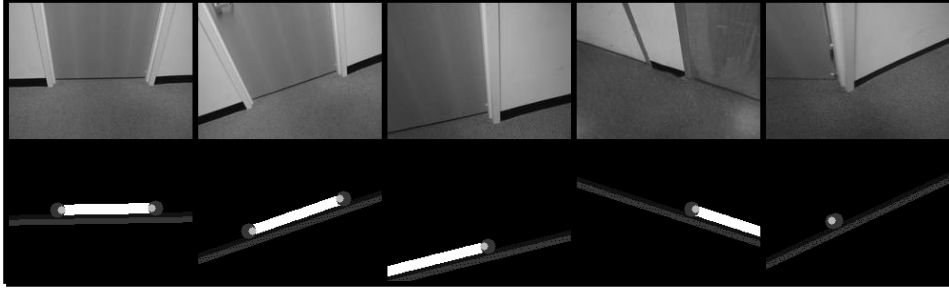
Fig. 10. CARDEA has a module for analyzing the door-floor interface, to detect exactly where the door frame is relative to its body, and whether the door has opened. This will be important when the robot has the ability to turn handles, so the robot can verify that the door is indeed opening. The Hough transform is used to find the strongest edge at \pm 45^\circ to the horizontal, and a Viterbi search is performed above this edge to find the best match for the door location, based on color information. The upper row here shows typical images on the floor-door interface, and the lower row shows the output of analysis. The circles denote the left and right edges of the door, and are connected by a dark line. The long light line denotes the floor line. The image on the right shows that when the door is open, this can be detected.
