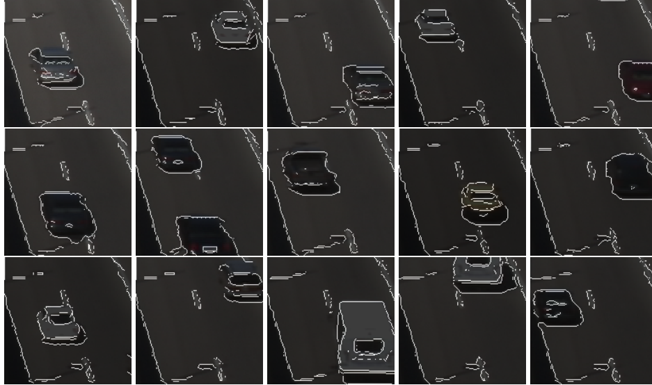
Figure 5: These results were inferred by the car model on images drawn from another road's traffic. The results required 40 candidates per node and 20 iterations of belief propagation.
