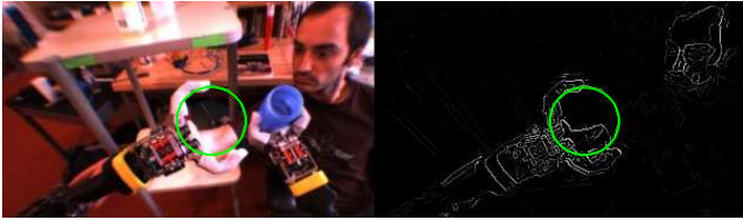
Fig. 4. The robot’s view as it transfers an object from its right hand to its left hand. The everyday environment includes the shelf, a person, natural lighting and a cluttered background. The edge motion (right) of the hand is used to estimate the location of the contact surface (green). This estimate is then used to visually servo the contact surface in the scene. In addition, the robot actively adapts its posture such that it can more easily view the controlled features.
