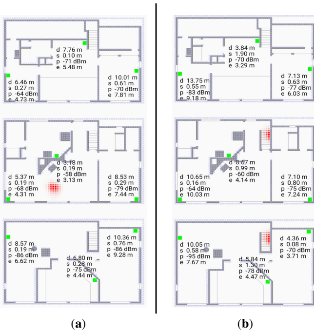
Fig. 11. Screen shots of application using Bayesian grid update method as a “heat map” (from video [30]). The voxels are 0.2 m on a side. The green spots are the responders. (a) (left subfigure) initiator in middle of the middle floor (b) (right subfigure) initiator on stairs between floors. Note that the paths between initiator and responder in most cases pass through one or more walls or floors. The Bayesian grid update method uses the observation model developed here.
