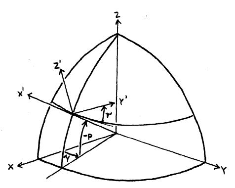
In this case we have the following sequence of rotations: roll-r about x-axis, pitch-p about y-axis and yaw-y about z-axis.
