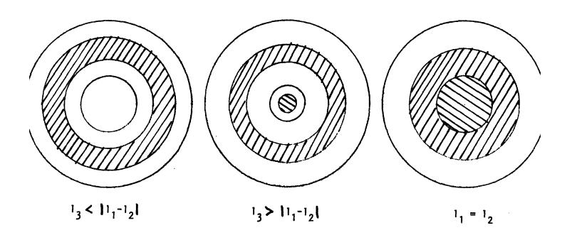
If  $l_3$  is less than  $l_1 - l_2$ , this new region is again an annulus, with inner radius  $l_3 + l_1 - l_2$  and outer radius  $l_1 + l_2 - l_3$ . The width of the annulus is twice the length of the shorter link minus  $l_3$ , its average radius is still equal to the length of the longer of link 1 and link 2. It is obviously a good idea to keep the third link short in order to achieve a reasonably large usable work-space.
