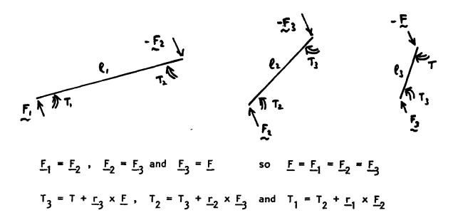
$$T_1 = T + (\underline{r}_1 + \underline{r}_2 + \underline{r}_3) \times \underline{F}$$
