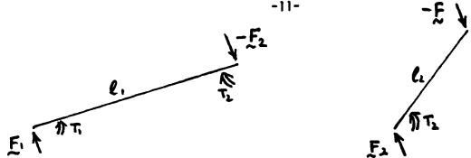
Note that the forces applied to each of the pin-joints in the device also have to balance as indicated in the diagram.
