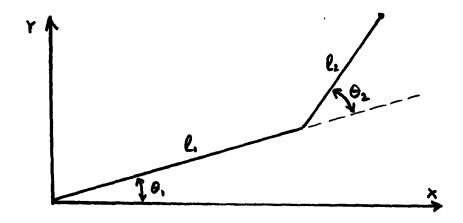
Given the two joint-angles, let us calculate the position of the tip of the device. Define vectors corresponding to the two links:
