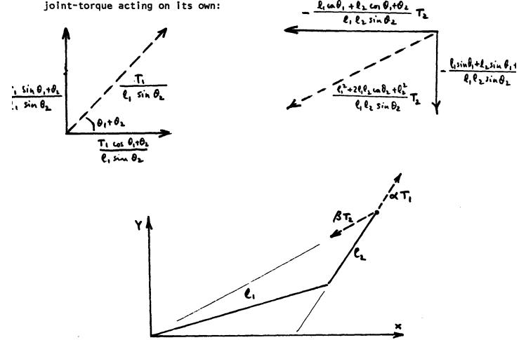
There are singularities in the transformation when  $\sin(\theta_2)=0$ , that is when  $\theta_2=0$  or  $\pi$ . Obviously when the links are parallel, the joint-torques have no control over the force component along the length of the links. Again we see the special nature of the boundary of the work-space.
