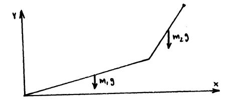
When there is no applied force at the tip we find that  $\underline{F}_2 = m_2 \underline{g}$  and  $\underline{F}_1 = \underline{F}_2 + m_1 \underline{g} = (m_1 + m_2) \underline{g}$ . Considering the torques we find:
