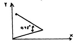
In the above diagram, if a torque is applied to joint 1, the push exerted on the end of link 2 is just enough to cause it to have an angular acceleration equal to that of link 1 and so  $\theta_2 = 0$ . Similarly if a torque is applied to joint 2 it will only cause angular accelerations in  $\theta_2$ .
