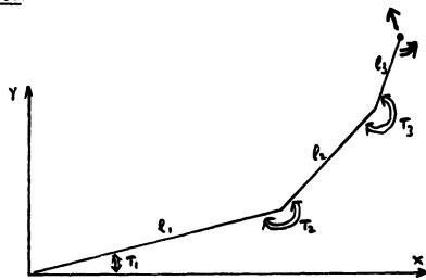
We have control over the three torques  $T_1$ ,  $T_2$  and  $T_3$  and would like to use these to apply force  $\underline{F}=(u,v)$  and torque T to the object held by the tip of the device. We do not want to consider motion of the manipulator now, so imagine its tip solidly fixed in place. We proceed by writing down one equation for force balance for each link and one equation for torque balance for each link.
