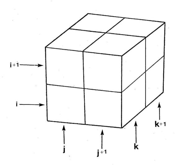
Figure 2. The three partial derivatives of image brightness at the center of the cube are each estimated from the average of first differences along four parallel edges of the cube. Here the column index j corresponds to the x direction in the image, the row index i to the y direction, while k lies in the time direction.
