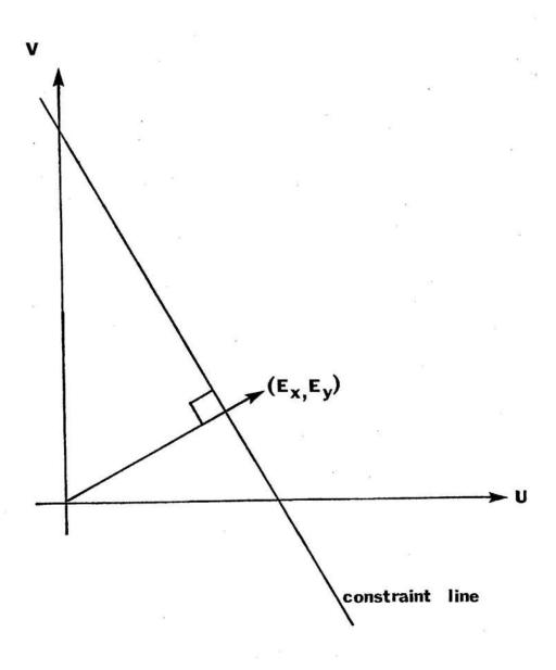
Figure 1. The basic rate of change of image brightness equation constrains the optical flow velocity. The velocity (u,v) has to lie along a certain line perpendicular to the brightness gradient vector  $(E_x,E_y)$  in velocity space.
