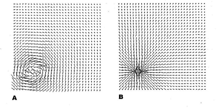
Figure 9. Flow patterns computed for flow around a line vortex and two dimensional flow into a sink. In each case the estimates after 32 iterations are shown.
